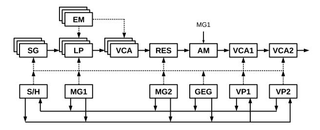
As you can see from the block diagram, there are many signal (solid) and modulation (dashed) paths between the various modules. The configuration is pretty flexible and can be reconfigured in the *Patch Bay*.
