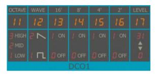
The *Wave* parameter determines the *weighting* of the respective harmonics in the mix – this way it is possible to create a staircase-shaped "Sawtooth" wave. Below are some examples of possible wave forms.
