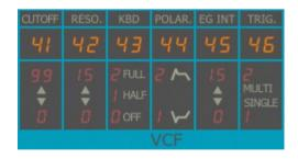
The VCF has its own DEG and offers positive or negative envelope modulation. Triggering modes of
