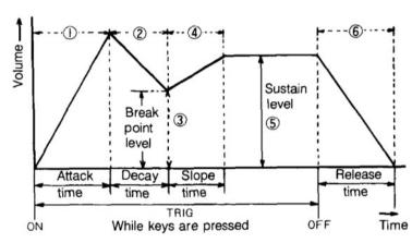
ADBSSR envelope – the diagram right is ripped from the original *Poly-800* Owner's Manual.
