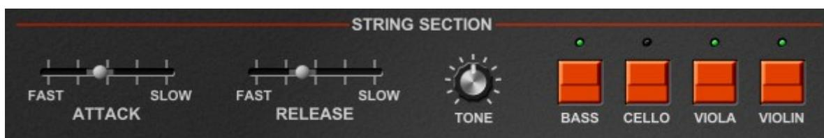
The "TONE" control shifts the frequencies of the internal formant filters for a "brighter" or "duller" sound of the instrument. Note that this control is not available on the original *Omni* and applies for all sections (*String*, *Synthesizer*, *Synth Bass*).
